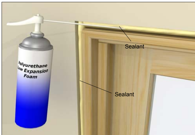
Figure 11 Apply low expansion foam between frame and rough opening
